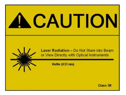
**Class 3R laser equipment, above MPE:** DANGER, Laser Radiation (or laser symbol), Avoid Direct Eye Exposure
