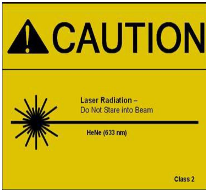
Figure 1: An example of signage required for general Class 2 Laser Equipment
