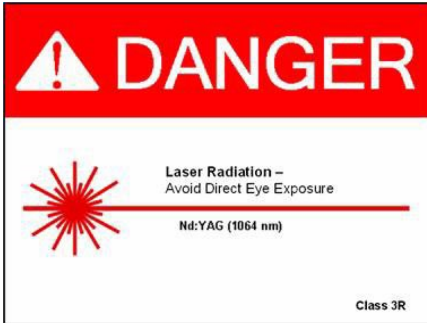
Figure 4: An example of signage required for Class 3R Laser Equipment, above MPE
