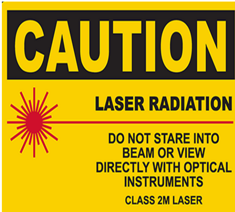
Figure 2: An example of signage required specifically for Class 2M Laser Equipment.
