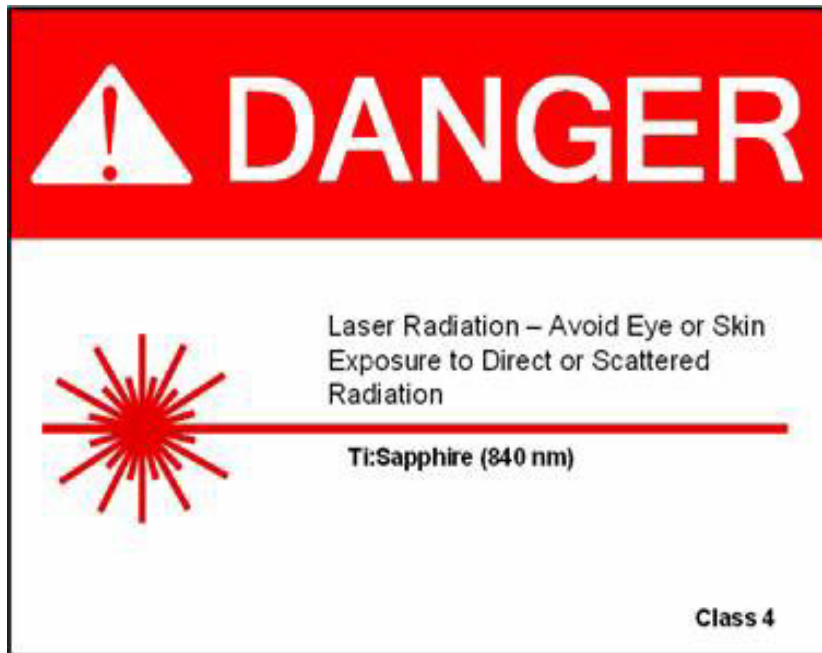
Figure 6: An example of signage required for Class 4 Laser Equipment
