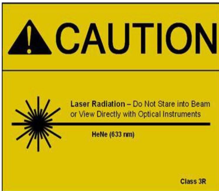
Figure 3: An example of signage required for Class 3R Laser Equipment, below MPE
